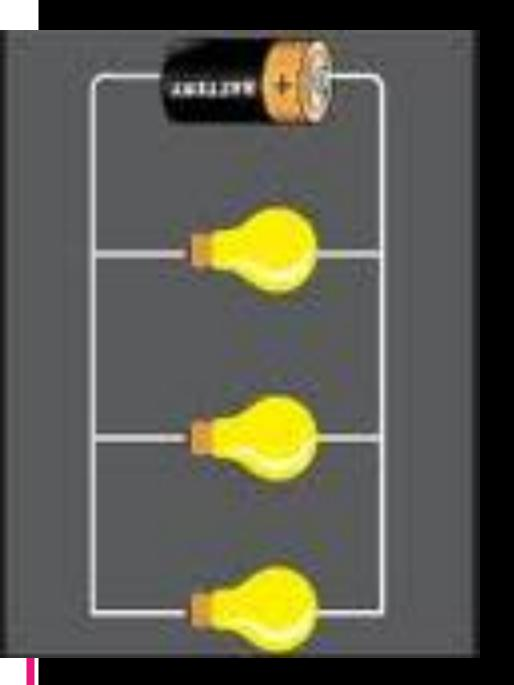
When bulbs are connected in **parallel**, the brightness remains the **same**. This is because the **voltage arriving at each bulb will be the same**.
