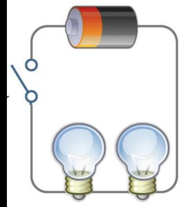
An extra bulb has been included. Do you think the bulbs will shine more or less brightly (once switched on)? Why? When bulbs are connected in **series**, the brightness decreases. This is because the **voltage splits** between each bulb.
