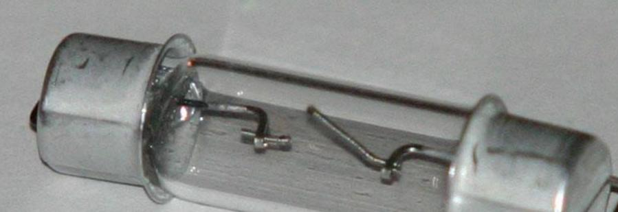
The fuse rating must always be slightly higher than the current flowing in the appliance. If less or equal, it will blow each time the appliance is switched on. If the fuse is much bigger than the appliance will overheat without blowing the fuse.
