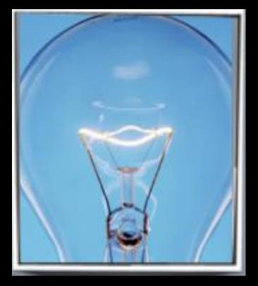
Do not forget that a filament bulb is made up of a small piece of metal that glows when electicity pass through it. If the metal (filament) is cut, then you do **not** have a complete circuit
