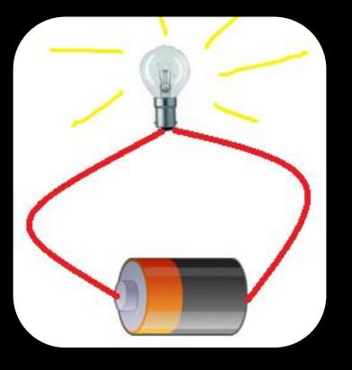
Electricity will only flow through a complete circuit.
