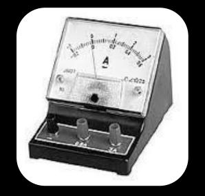
The ammeter measures current in amps. The symbol for amps is A.
