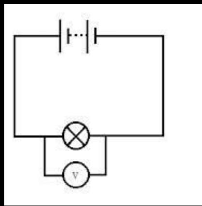
It is placed before or under the bulb, in a separate loop.
