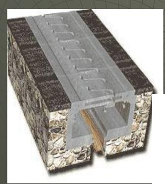
Bridges have expansion joints and rollers under them so that when it's hot the bridge doesn't buckle.
