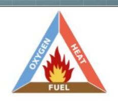
Sand covers the fuel and keeps oxygen away, Can be used on any fire.
